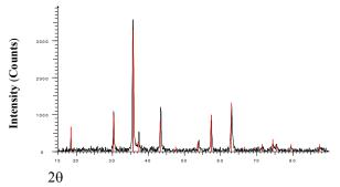
Figure 1. X-ray diffraction pattern of NiAl0.5Fe1.5O4 nanoparticles.
