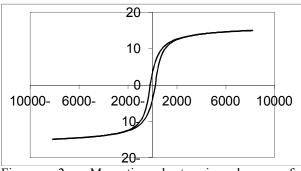
Figure 2. Magnetic hysteresis loop of NiAl0.5Fe1.5O4 nanoparticles.
