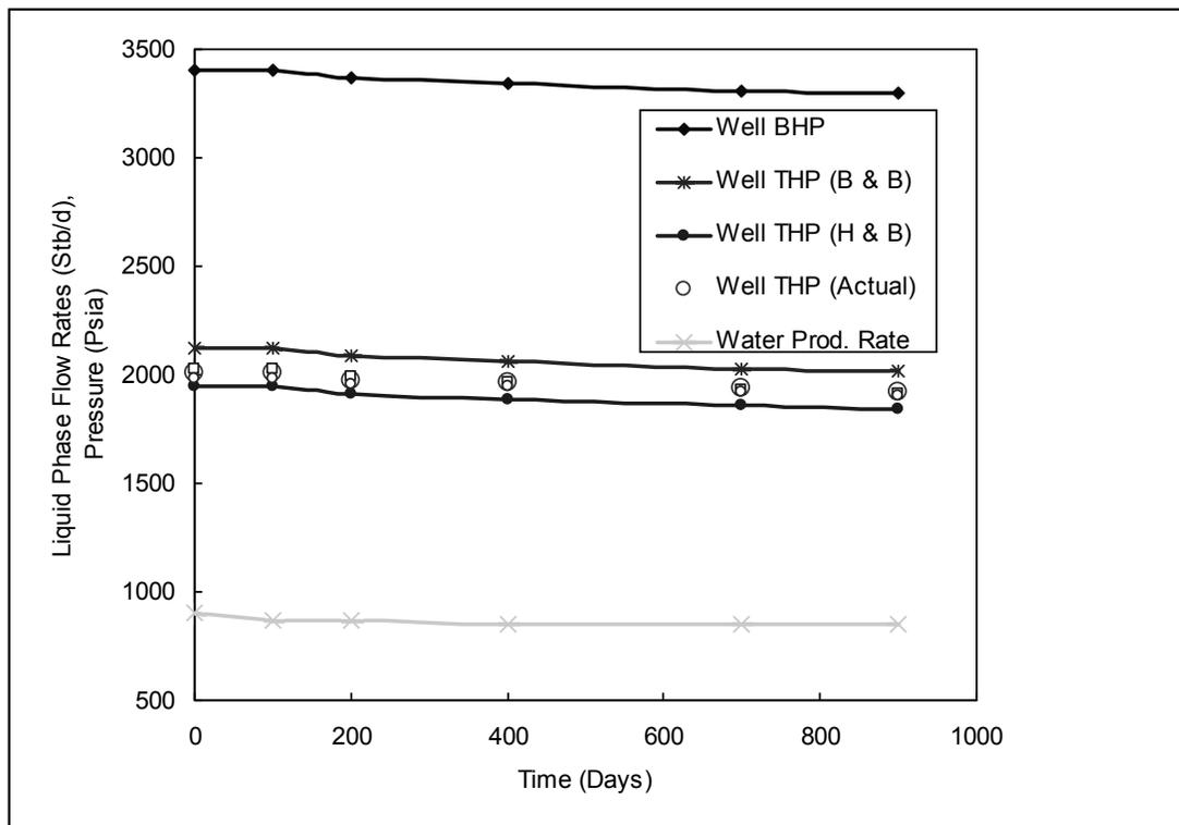
Figure 5. Water producing well production profile
