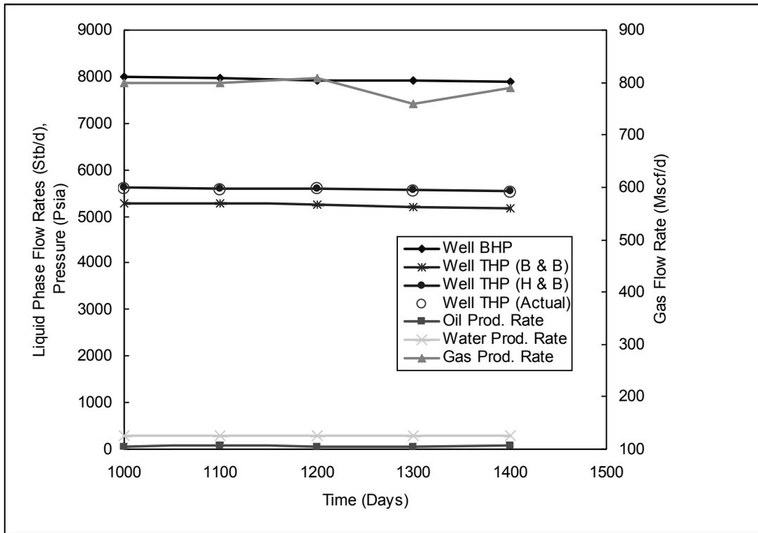
Figure 4. Gas well (also producing some condensate) production profiles
