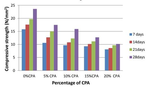
Figure 5: Compressive strength of CPA concrete at different curing days
