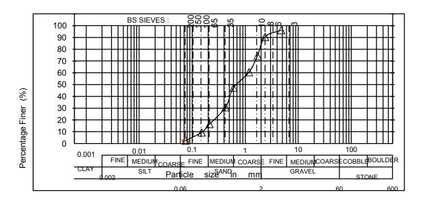
Figure 2: Particle size distribution for the sharp sand
