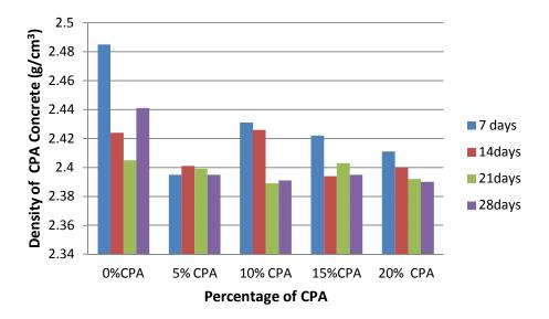
Figure 4: Density of CPA concrete at different curing days
