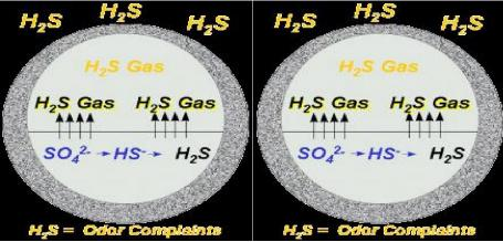
As you see in (Fig. 1),  $h_{2^s}$  Produced From the Surface of Wastewater Rises, and is Mixed With Headspace Air of Collection Networks and Sulfuric Acid is Formed;
