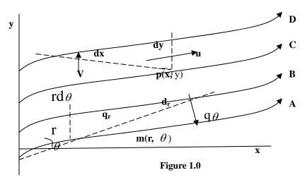
The figure 1.0 shows a representative plane for two-dimensional flow, with four streamlines denoted by the letters A, B, C, D. the whole pattern may be shifted
