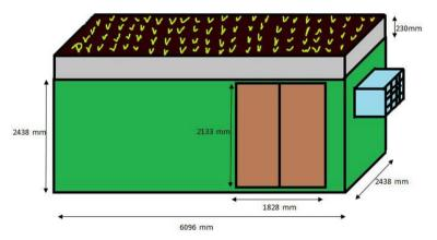
Figure 3. Diagram of experimental green roof [15].
