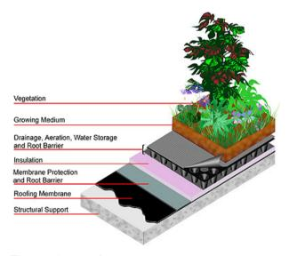
Figure 1. Green roof cross section.
