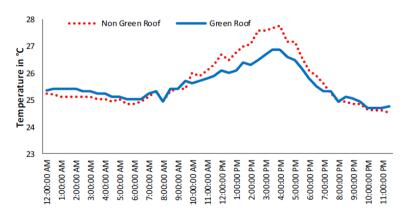
Figure 4. Temperature profile of both green roof and non-green roof systems in summer (26th February 2013).
